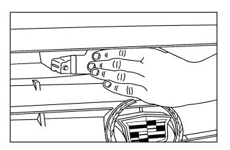
Then go to the front of the vehicle and find the secondary hood release lever. The lever is located under the front edge of the grille near the center. Move the release lever to the side and raise the hood.
